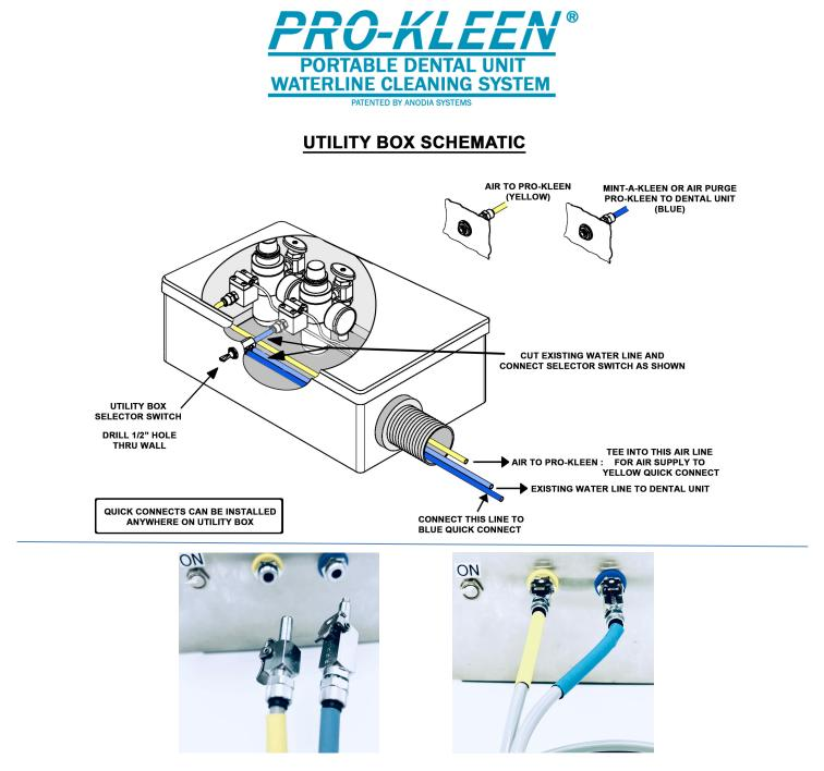
Color Coded (Yellow and Blue) Male Quick Disconnects on PRO-KLEEN Allows the Operator to Match the Female Color Coded Quick Disconnects on the Utility Box. The Yellow Quick Disconnect is for Air which Pressurizes the PRO-KLEEN. The Blue Male Shut Off Quick Disconnect Prevents Air or Mint-A-Kleen from being Injected until This End is Inserted into the Female Quick Disconnect on the Utility Box. This Blue Coded Line is the Route for Air and Mint-A-Kleen into the Dental Unit's Water Line.
